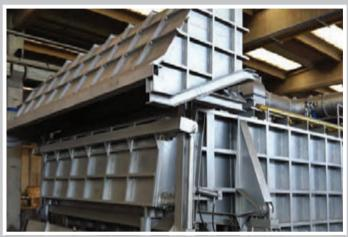
Thanks to our expertise, the furnaces are manufactured to burn with different type of fuels (natural gas, LPG, Fuel oil). The heating can be made with common burners, radiant, self-healing, recovering and hot air.
