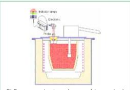
PLP non contact probe used to control the maximum level in a furnace
