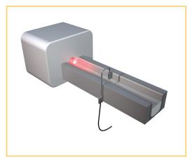
The OFG-285 consists of a main unit with a safety circuit and a swing arm conduit to an electrode head. The main box can be mounted to brackets 50 mm (2") outside a launder. The electrode head is to be swung over the molten metal and leveled so that the ends of the electrodes hit just above the maximum allowed level in the launder. The electrode head can be swung out from the launder during maintenance.
