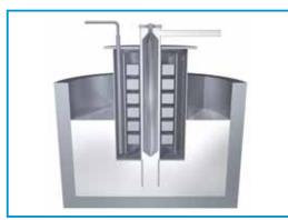
Electromagnetic Pumps - available in configurations withstanding up to 800°C; suitable for zinc, lead and tin applications - other metals at request.
